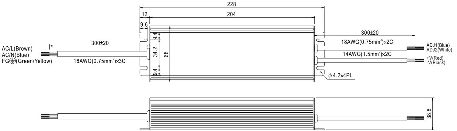
※ IP67 rated. Output constant current level can be adjusted through output cable by connecting a resistor or 1 ~ 10Vdc or 10V PWM signal between ADJ1 and ADJ2.
