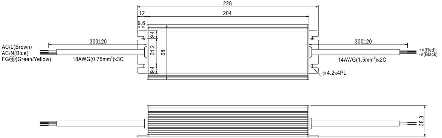
※IP67 rated. Cable for I/O connection.
