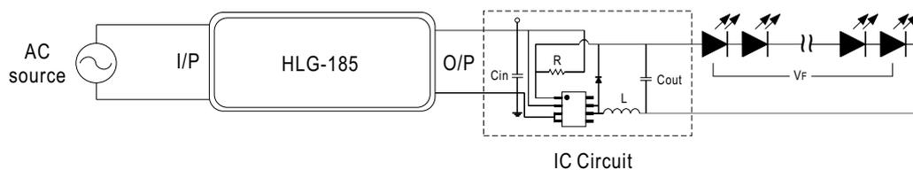
◎ **Dimming application connection diagram (for turning the lighting ON/OFF) :**
