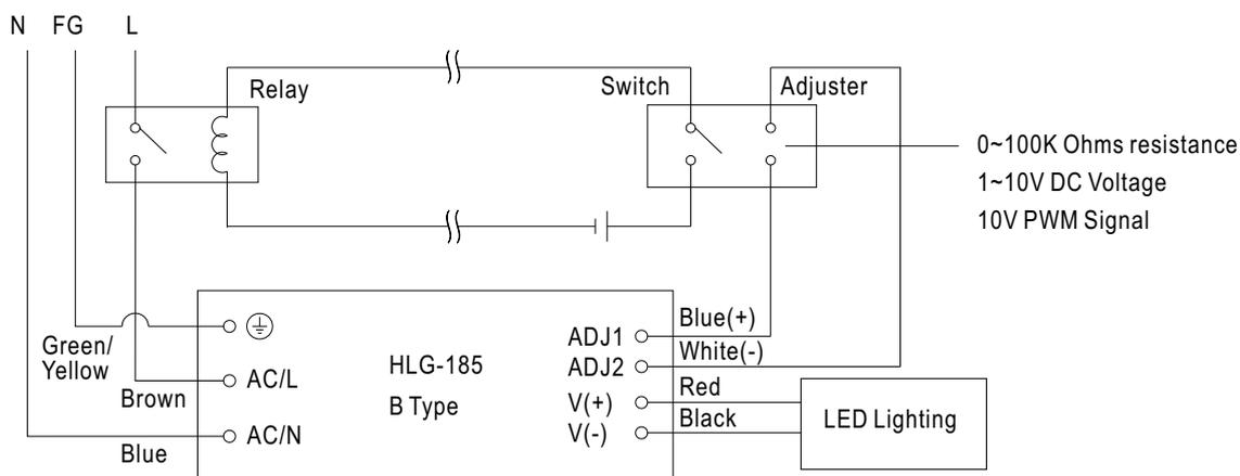
Using a switch and relay can turn ON/OFF the lighting.
